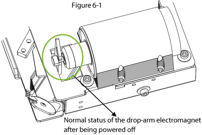
Normal status of the drop-arm electromagnet after being powered off
