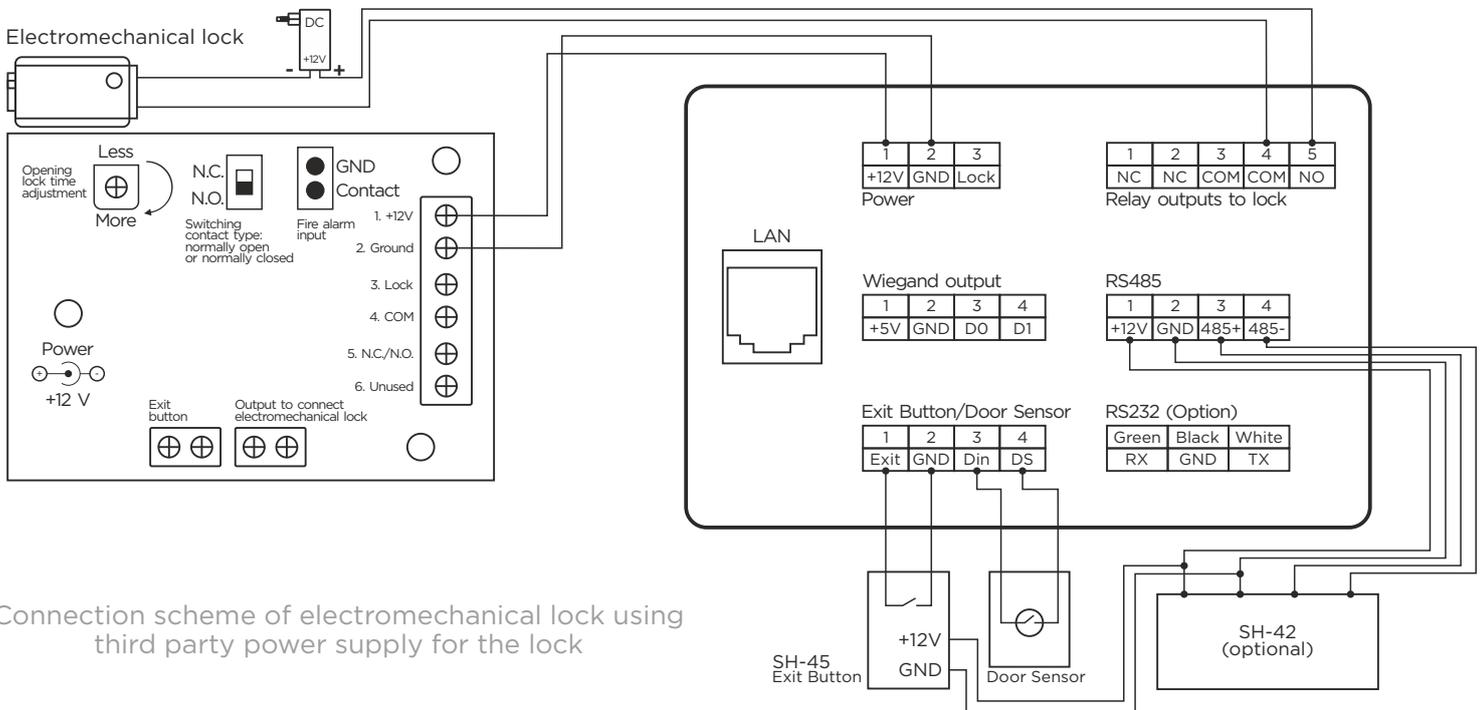
Connection scheme of electromechanical lock using third party power supply for the lock
