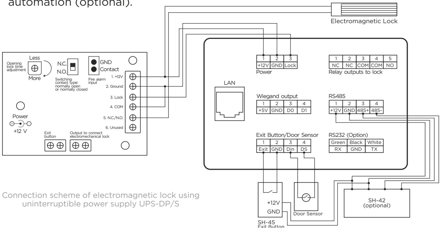
Connection scheme of electromagnetic lock using uninterruptible power supply UPS-DP/S
