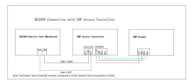
**Note:** The Reader1 and 2 of Inbio260 Controller corresponds to LOCK1, Reader3 and 4 corresponds to LOCK2.
